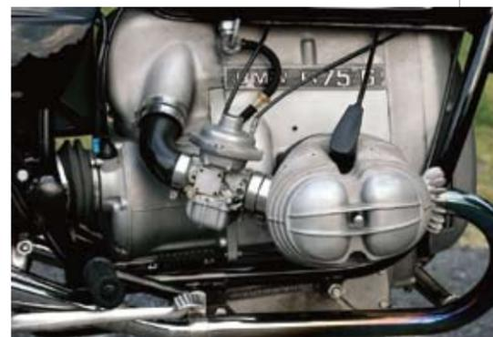
Gentleman's express: Bill Kniegge's revamped Boxer is a serious cruiser. Cylinders and pistons from an R100 boost the original R75's displacement from 745cc to 980cc, while modified R90S front forks with dual disc brakes maintain control.
