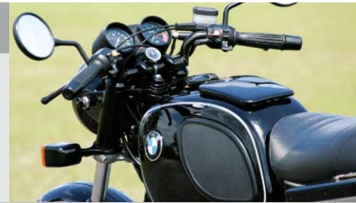
are powder coated black to match the tank and laced with stainless spokes. After a trip to the powder coater, Bill is soon bolting on a black swing arm, both triple clamps and the handlebar mounts. The fenders, headlight and side panels are painted with black lacquer, and the headlight rim and gas cap get treated with black chrome.
